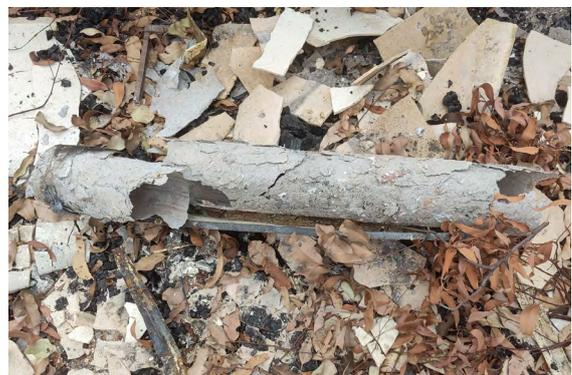
Figure 7 Fire damaged asbestos cement flue.
