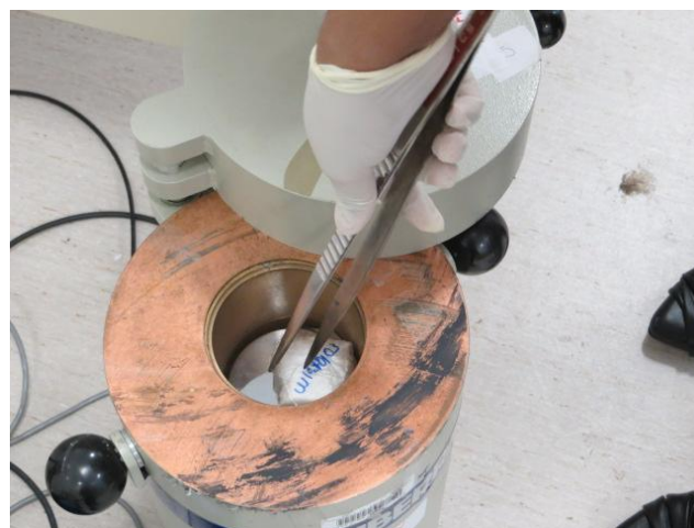
Figure 12 A wipe swab being placed in equipment for analysis in the Radiation laboratory.
