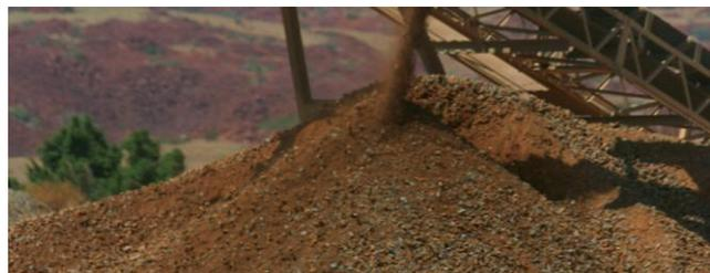
Photo: Cracker dust is created during the crushing of aggregate. Source: [Department of Mines and Petroleum](#)
