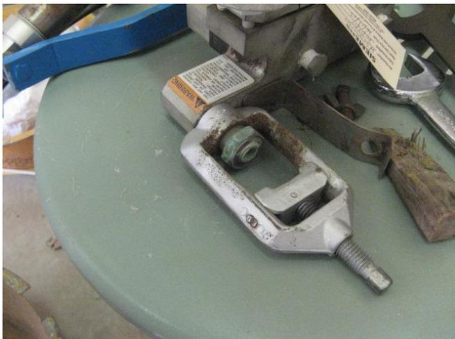
Photo: Corroded bolt that contributed to the chlorine gas leak.
